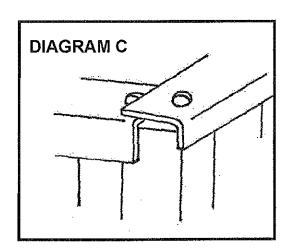
4. Now same procedure as 3. with the last side wall, making sure panel overlaps and split pin is placed through both holes. Then carry out the same procedure for the door frame.
